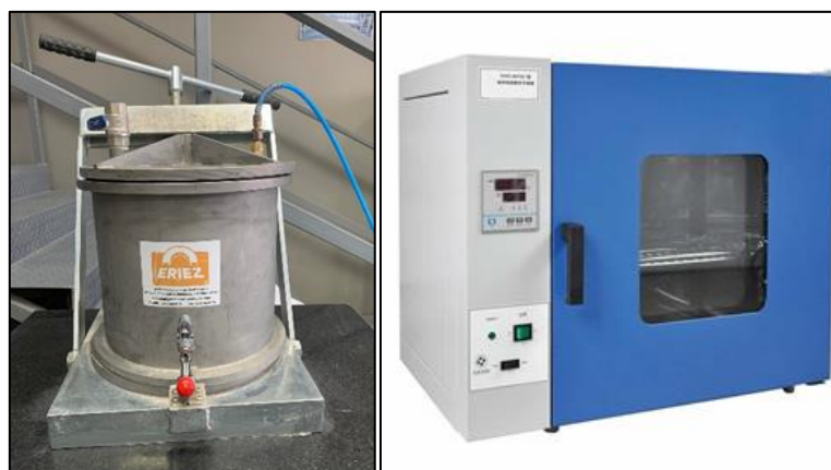
Figure 13. (a) MascaLab Filter Press and (b) Lichen Technology Electric Blast Drying Oven
