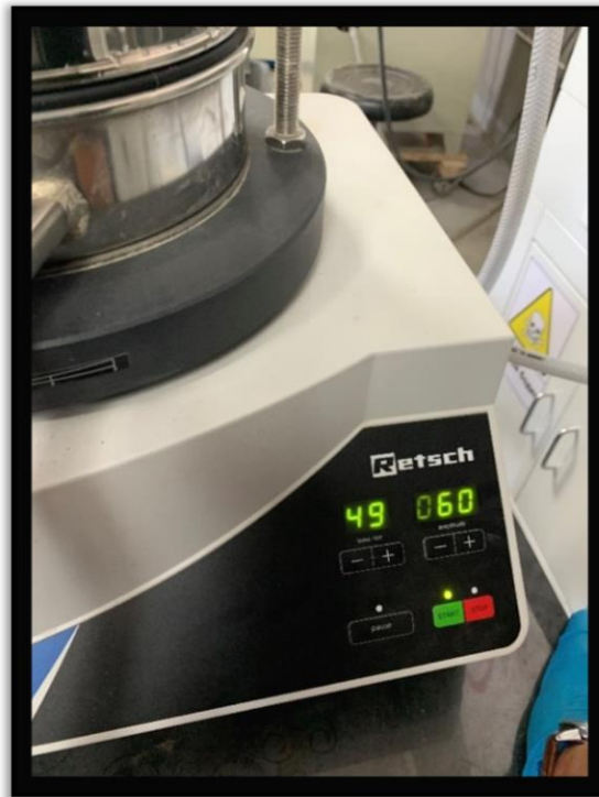
Figure 11 Wet sieving set up
