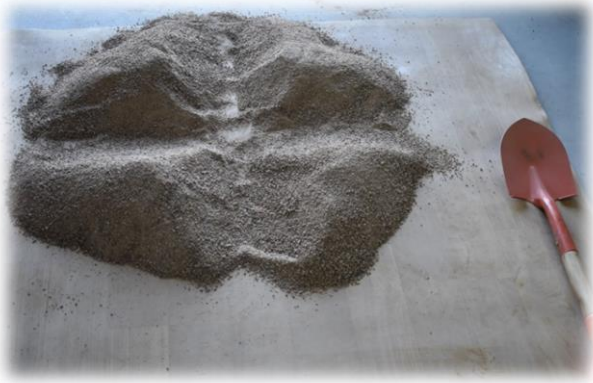
Figure 4-4 Mark the four quarter top of the ore
