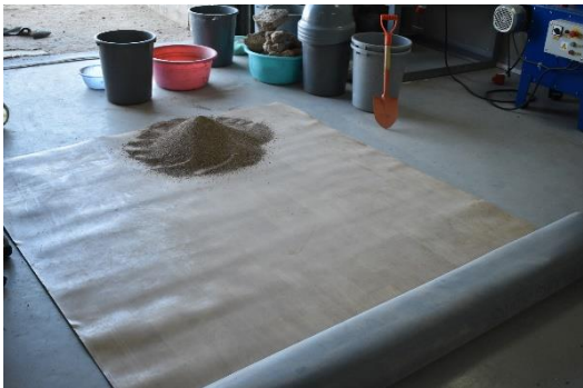
Figure 4-2 Prepare for using coning and quartering method
