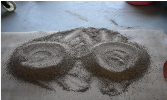
Figure 4-5 After Marking the removing opposite quarter the blending again
