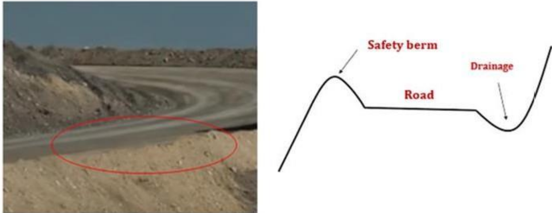
Figure 10 Scheme of safety berms and drainage [11].
