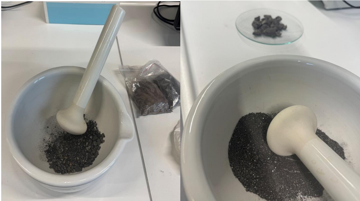
Figure 8: Crushing of sphalerite mineral sample using mortar and pestle.
