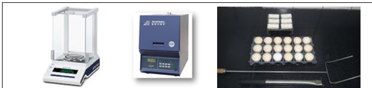
Picture 7.2-1 Ash content analysis tools (left side: weight measurement, incinerator, and crucible)
