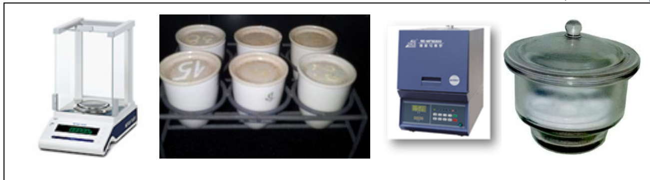
Picture 7.2-2 Volatile matter content analysis used equipment (Left side: weight measurement, crucible, laboratory incinerator, and desiccator)
