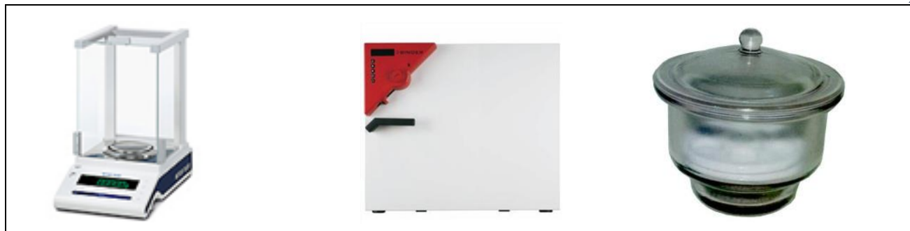
Picture 7.2-3 Analytic moisture content analysis used equipment (Left side: weight measurement, laboratory drier, and desiccator)
