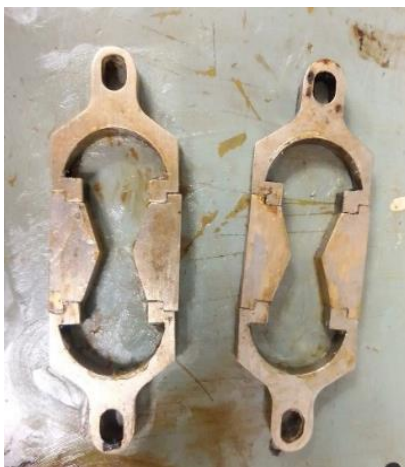
Figure 14 Ductilometer sample cast
