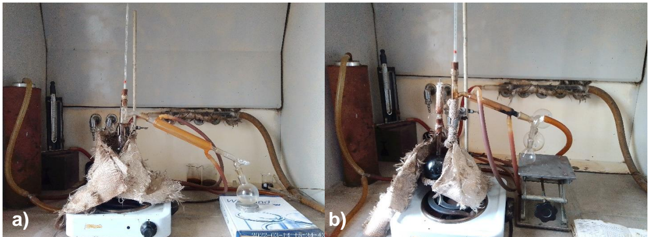
Figure 25 a) Atmospheric distillation, b) Vacuum distillation
