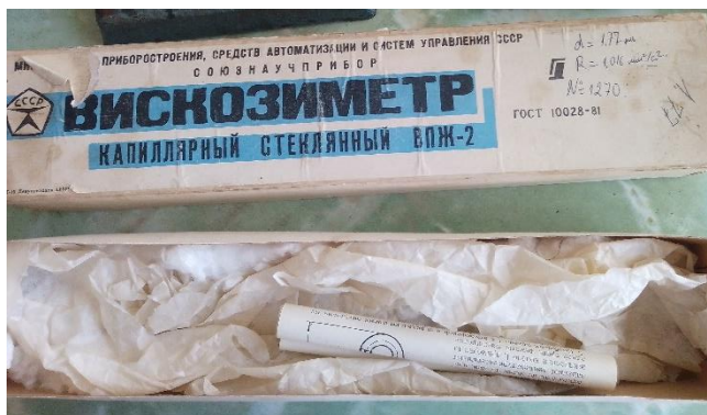
Figure 9 Used Viscosimeter with constant 1.016
