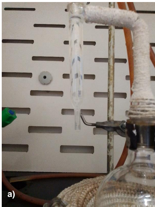
Figure 6 a) Dean-Stark glassware, b) Dean-Stark apparatus
