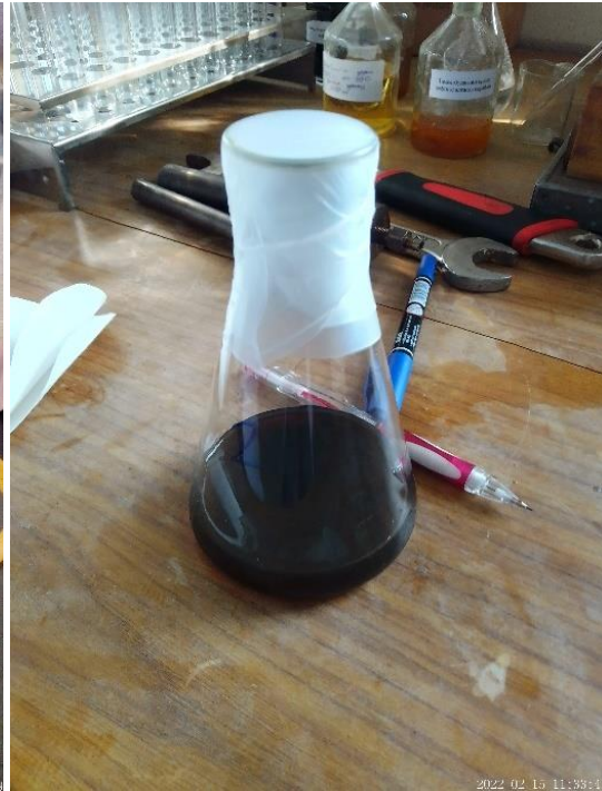
Figure 18 Dissolving crude oil in n-hexane, 1:40
