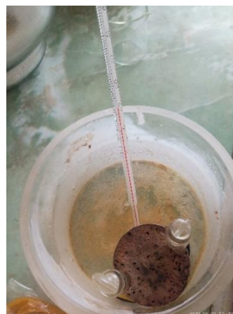
Figure 7 pycnometers in a 20C water tub
