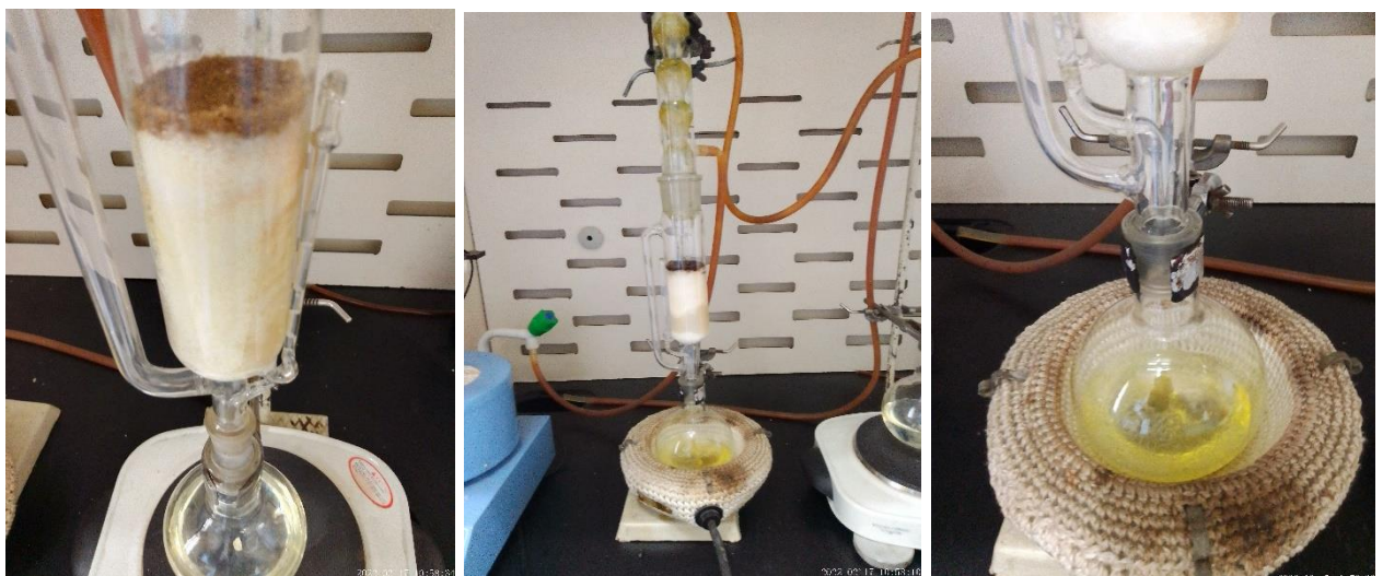
Figure 22 Extraction of oil constituents with activated silica gel
