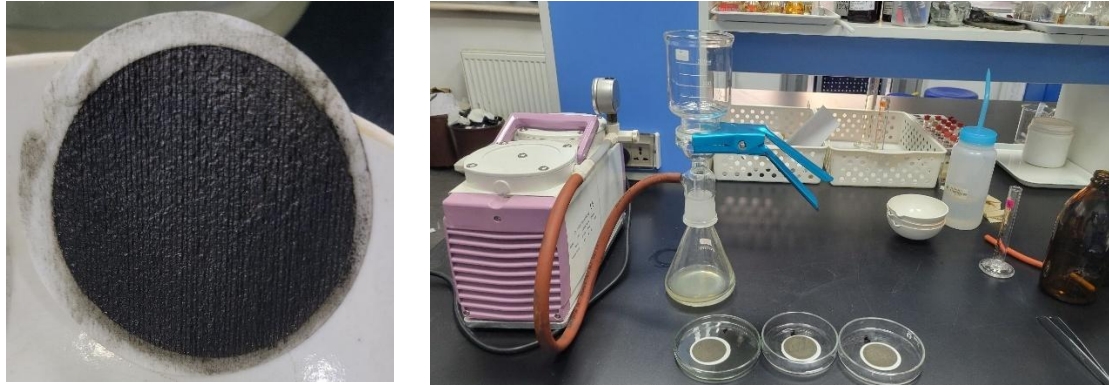
Figure B. 2. Filtration Setup and Glass Fiber Filter Paper Used for TSS Measurement
