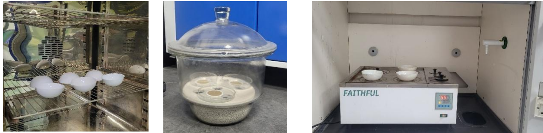
Figure 6. Apparatus Used for Total Solids Analysis
