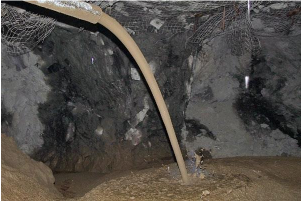
Figure 3. Process of hydraulic backfilling (13)
