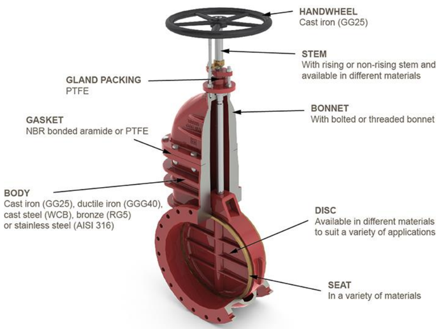
Figure 4.7. A typical gate valve (manually operated)
