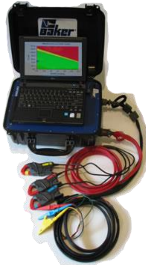
Figure 27. Voltage measurement by Baker EXP3000 Explorer in the field
