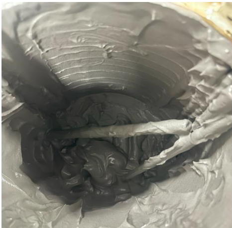
Figure 35 Condition in rod mill chamber of L:S of 0.4:0.6
