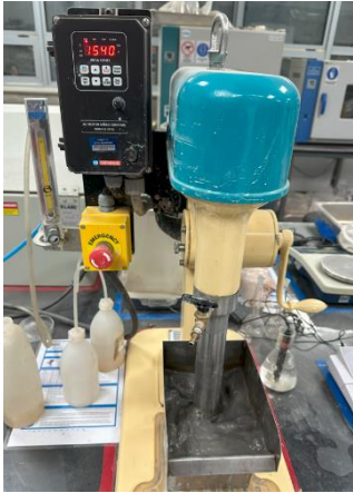
Figure 25 Metso D12 Laboratory Flotation Machine
