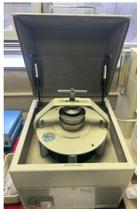
Figure 18 Laboratory Vibration Cup Mill
