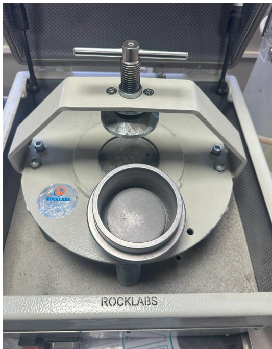
Figure 18 Laboratory Vibration Cup Mill
