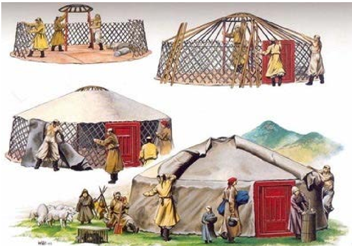
Figure 2. Constructing process of a ger
