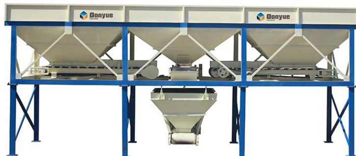
Figure 2. Construction material dosing machine
