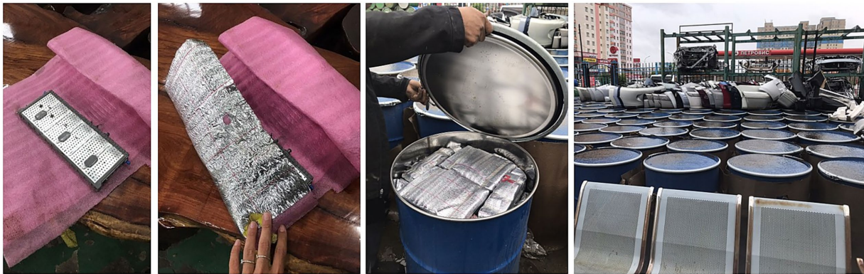
FIGURE 11 Preparation of NiMH modules to be exported. Source: Prates et al. (2023). (authors' own archive).
