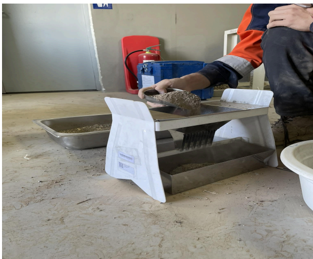
Figure 2.1.3: a) Process of using a riffle splitter to divide crushed feed into portions with the same particle size distribution, b) Riffle splitter
