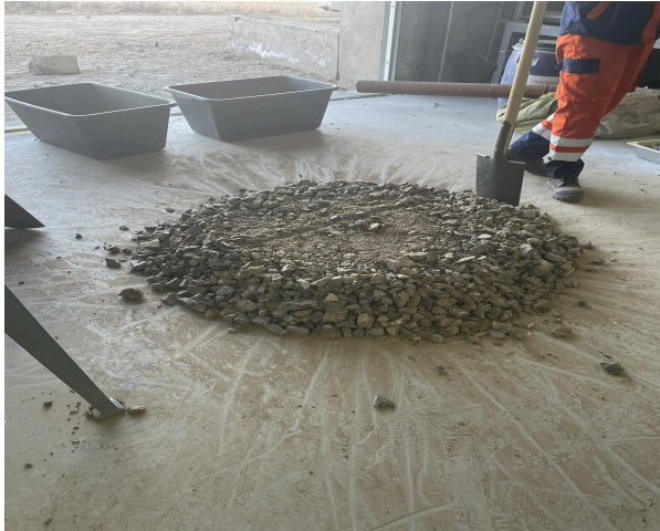
Figure 2.1.1 - Zinc Ore Feed Preparation Using the Coning and Quartering Method
