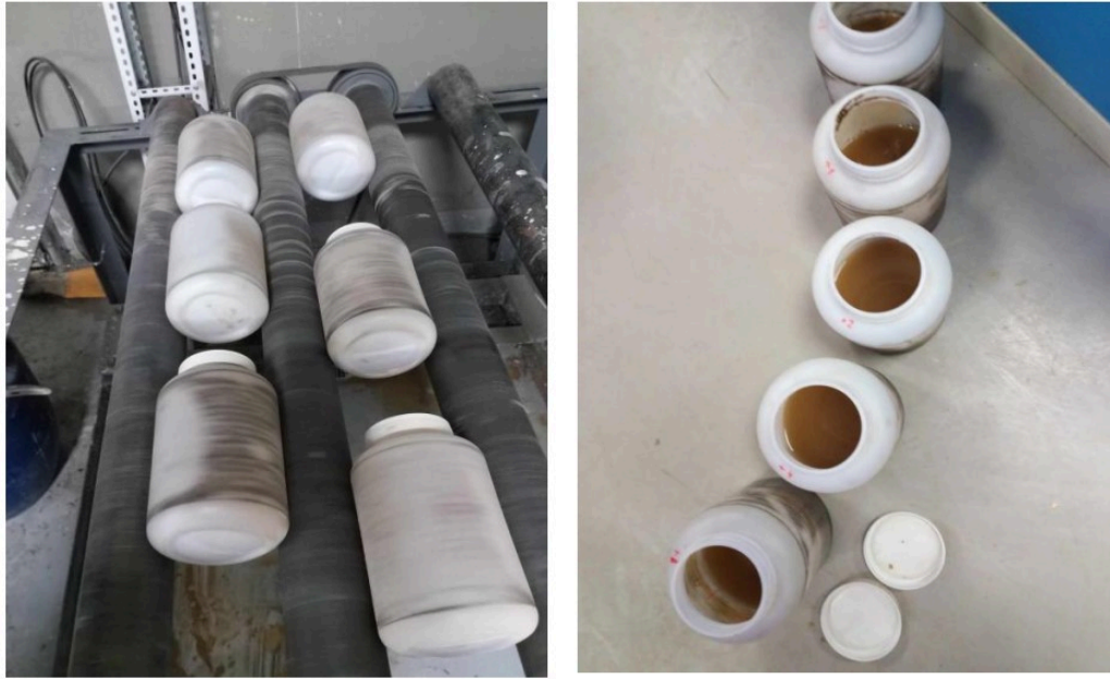
Figure 3.5.2: Bottle Roll Leaching Procedure
