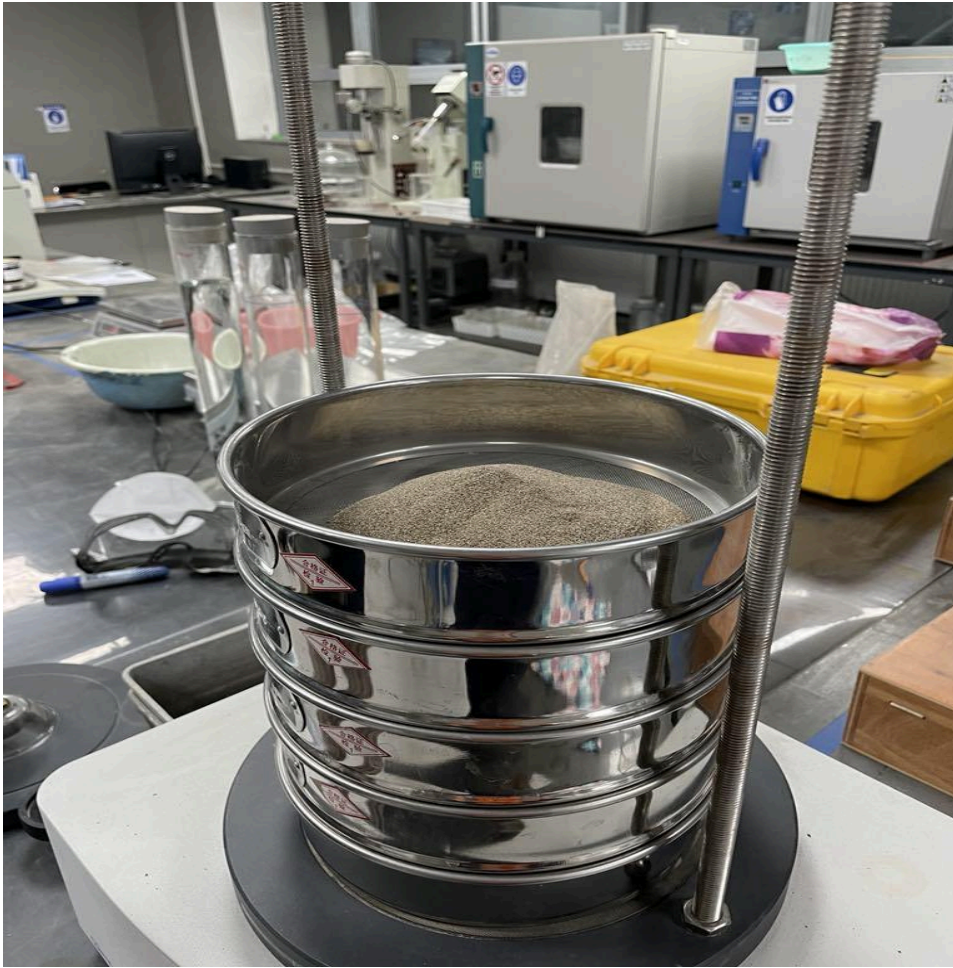
Figure 3.2.4 Screen Analysis for the product of rod milling
