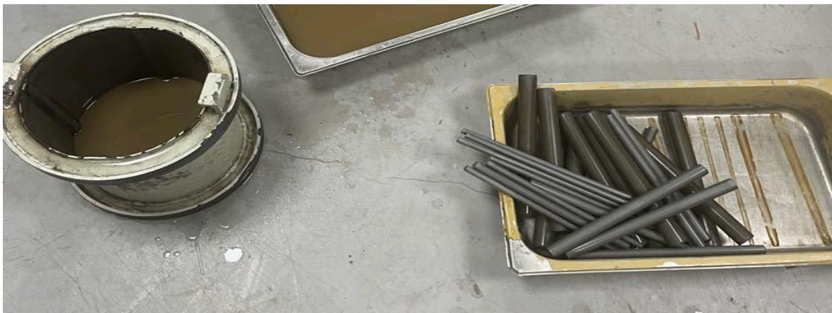
Figure 3.2.3: Rod Mill Container and Rod Mill Used in the Rod Milling Process
