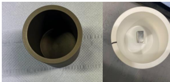
Figure 6: a) Graphite crucible b) Boron Nitride crucible
