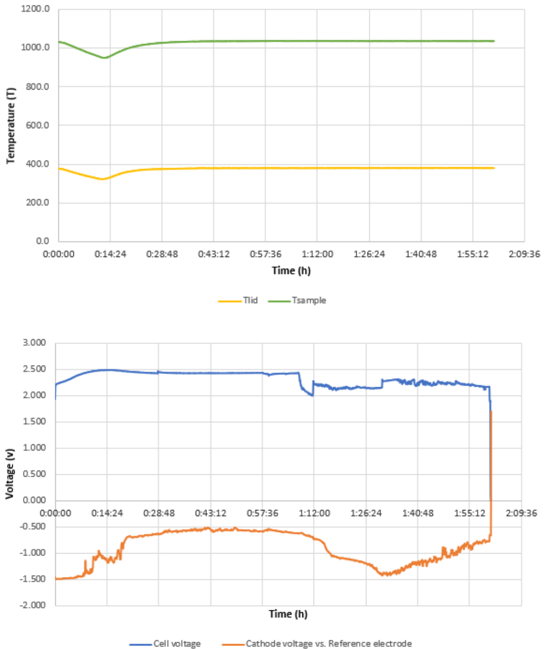
Figure 28: (a) Lid and internal cell temperatures measured during electrolysis. (b) Cell voltage and cathode potential vs. tungsten reference electrode over time
