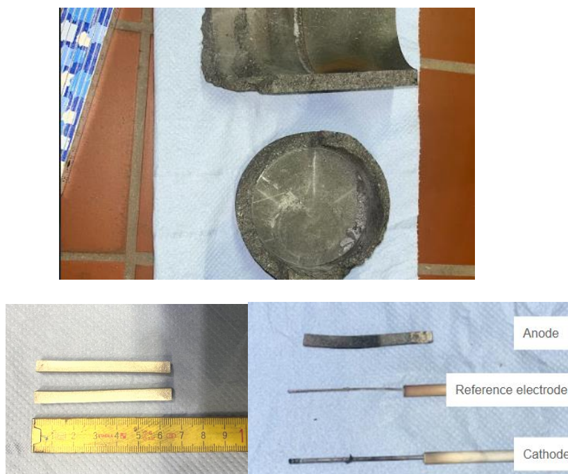
Figure 26: After 2 h of electrolysis a) broken graphite crucible used in the experiment; b) inert anode before electrolysis; c) post-electrolysis anode, cathode, and tungsten reference electrode.
