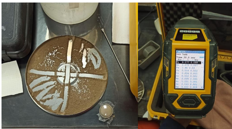
Figure 19 Soil sample preparation for XRF analysis
