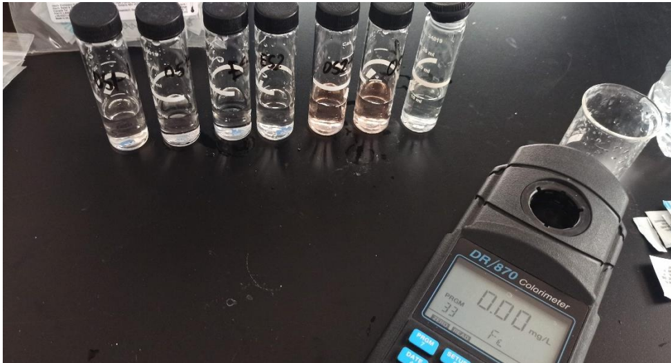
Figure 18 Measurement of iron concentration using FerroVer
