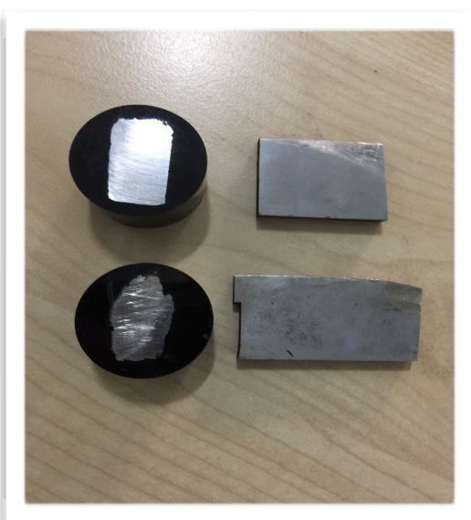
Figure 73: Embedded hardox pieces
