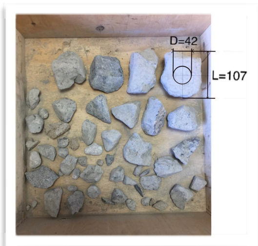
Figure 69: Comparing ideal mean diameter with actual particles
