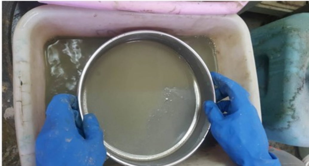
Figure 15 Washing grinded ore with 74 micrometer sieve
