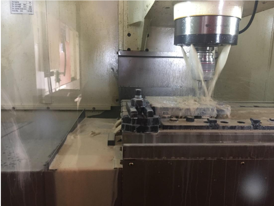
Figure 2523 – Corner drilling operation
