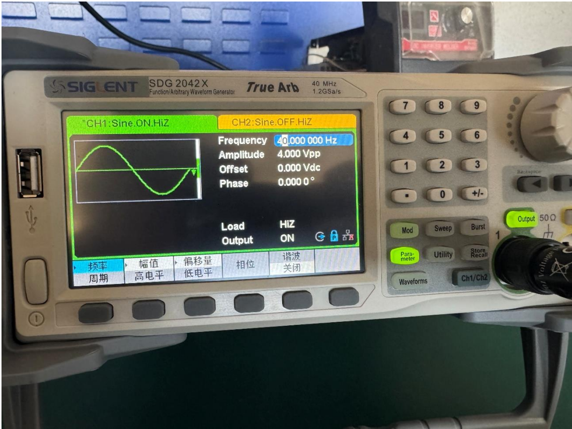
Figure 47. Function generator creating a 40Hz sinewave
