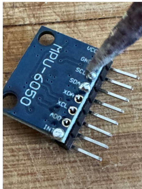
Figure 45. Soldering MPU6050 for in use process
