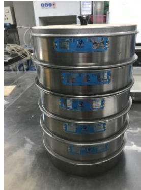
Figure 3. 7 Laboratory stainless steel sieves utilized in the experiment
