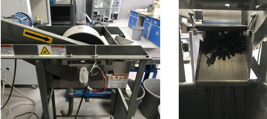
Figure 3. 11 Wet Low-Intensity magnetic separation
