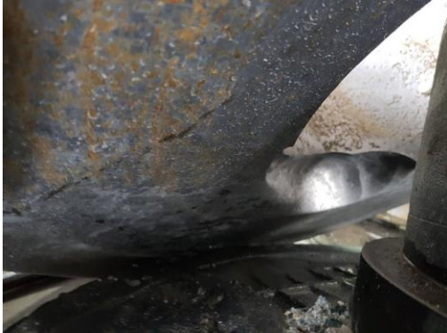
Figure 60: Regular cover plate with similar wear
