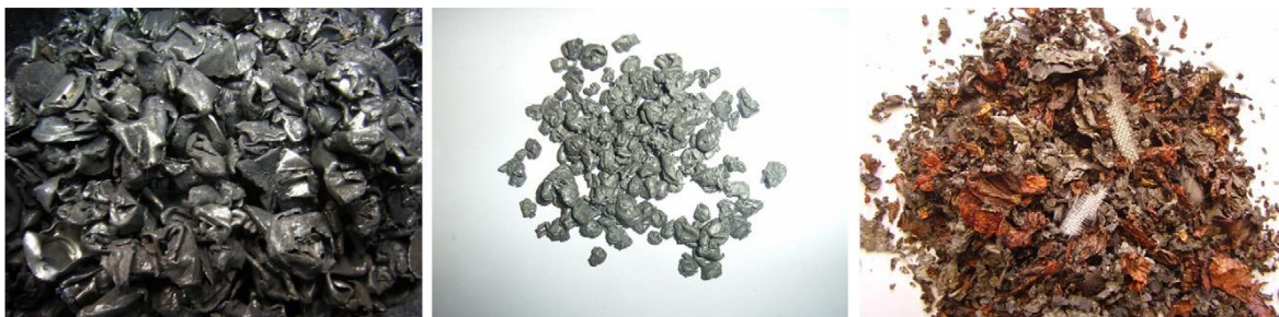
Figure 18 Metal containing material fractions (from left to right; iron-nickel fraction, aluminum fraction, electrode foil fraction) (18)
