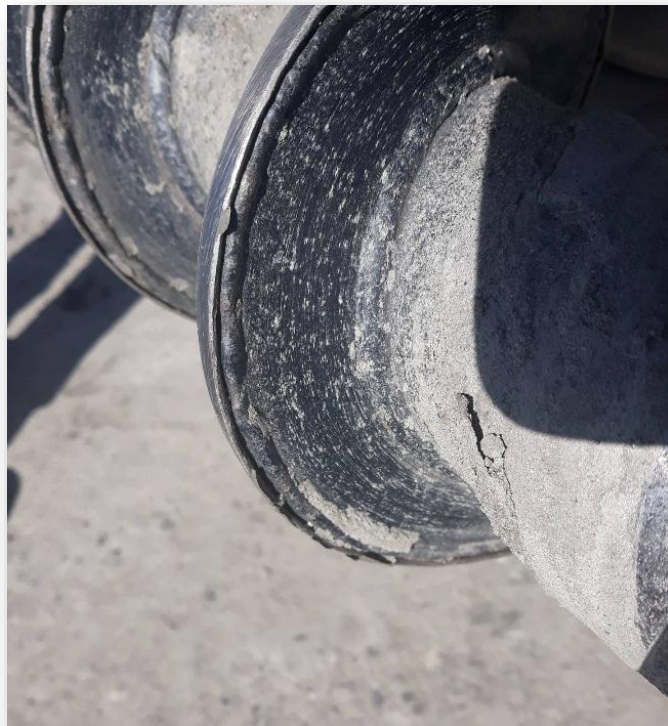
Figure 3. 3 – Welded drilling rod
