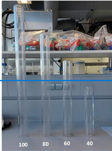
Different height of flotation column
