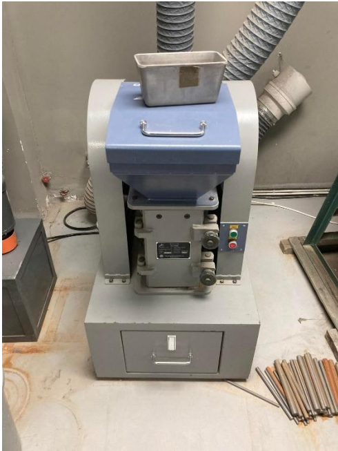
Figure 22. 5E-JCA jaw crusher to comminution size of -6mm
