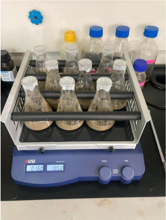
Figure 23. All 9 samples were prepared and put on an linear shaker at 150 rpm
