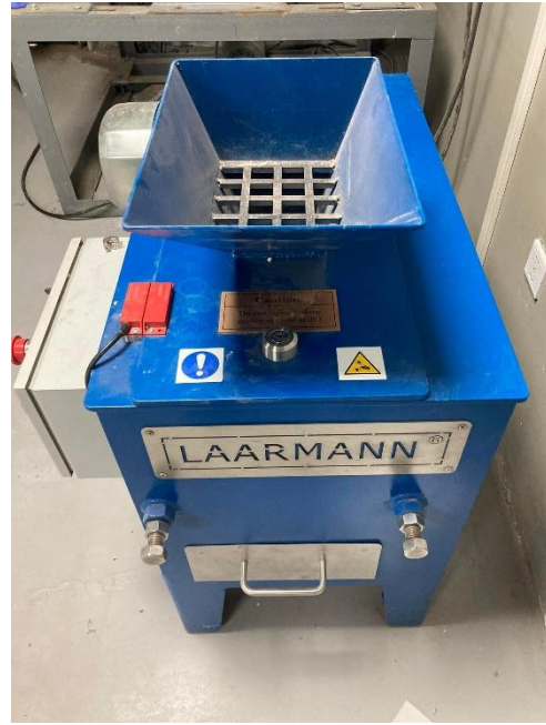
Figure 21. Roll crusher to comminution size of -2mm
