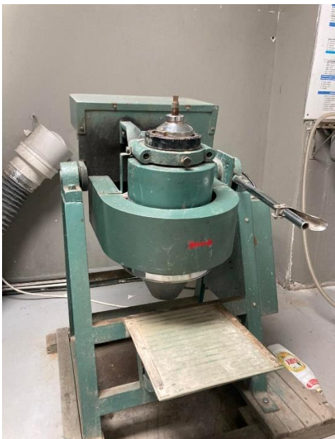
Figure 20. Rod miller used in this study for comminution size of -75 micrometer
