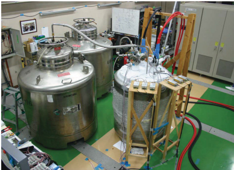
Figure 4.15 The illustrative topology of an SMES system. The liquid helium is contained in the two tanks on the left, while the tank on the right contains the superconducting coil. Source: Nielsen, 2010 [176]. Reproduced with permission of K.E. Nielsen.
