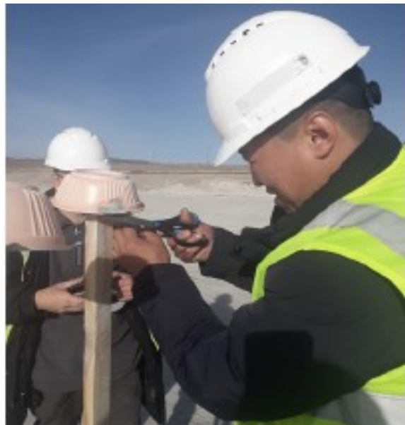
Photo 16: Dust-collecting pads secured by tape so that they are not in contact with the wall of the container
