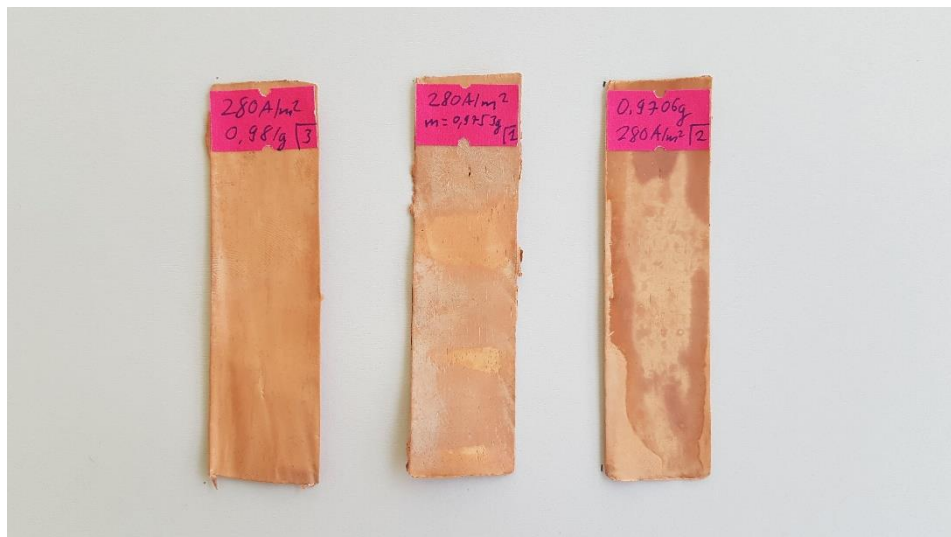
Figure-26 Cathode sheet of electrowinning experiments with current density at 280A/m 2
