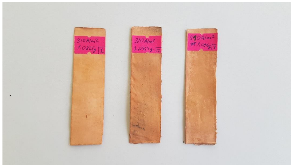
Figure-27 Cathode sheet of electrowinning experiments with current density at 310A/m 2
