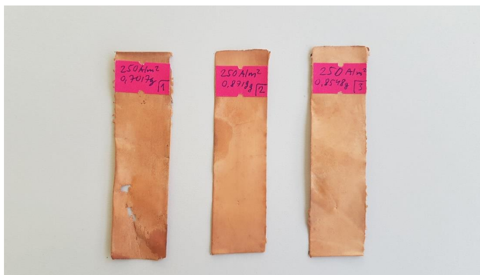
Figure-24 Cathode sheet of electrowinning experiments with current density at 250A/m 2
