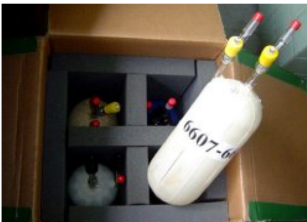
Figure 6. (a) (b) Process of GHG sampling (c) Shipping box used for transporting samples to the NOAA
