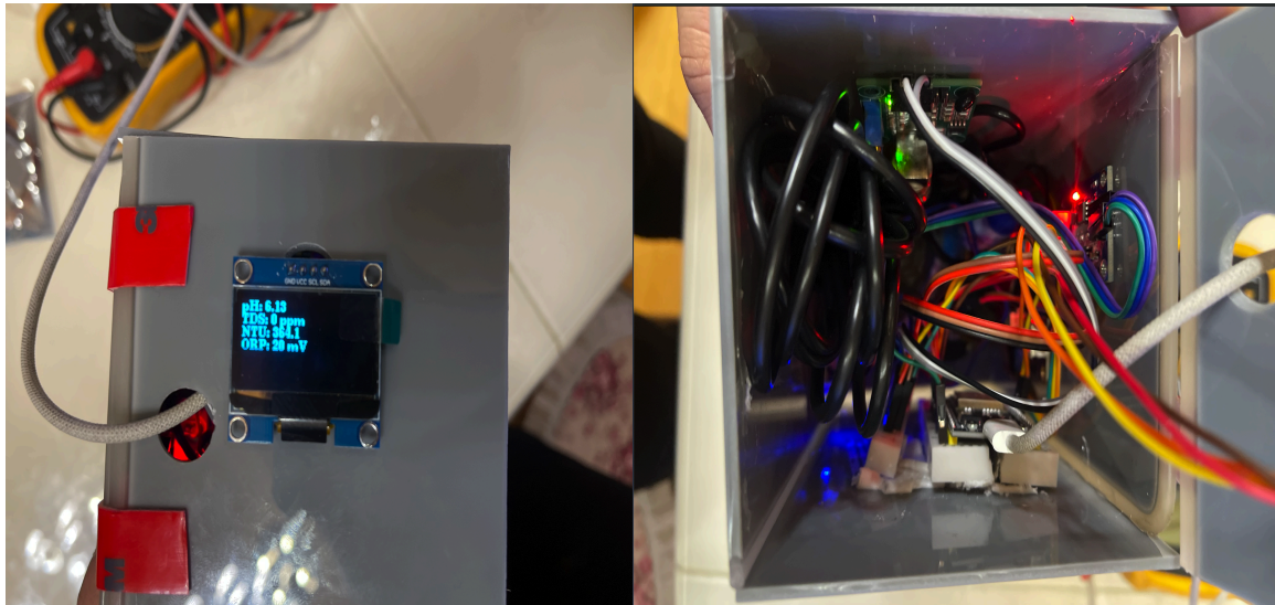
figure 17. Assembled prototype showing OLED display output and internal wiring
