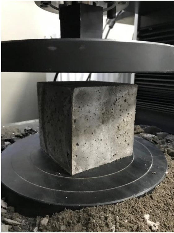
Appendix 22 Before compression test
