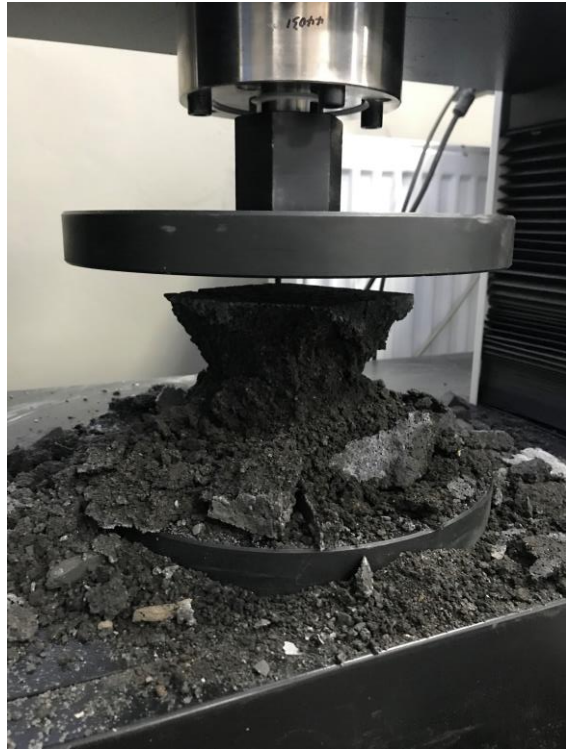
Appendix 23 After compression test
