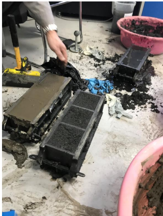
Appendix 18 Molding process of mix
