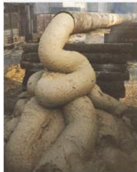
Figure 14 Mine cycle comparison between slurry and paste backfilling Figure 15 Paste backfill (13)
