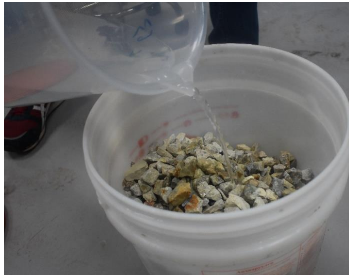
Figure 17: 10% of sulphuric acid solution mixing with ore
