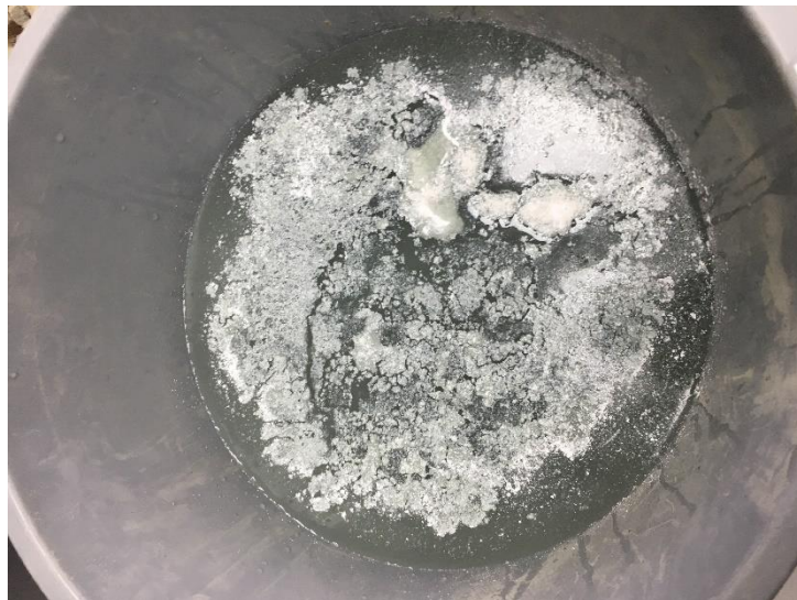
Figure 22: The leaching liquid residue is neutralizing by calcium hydroxide
