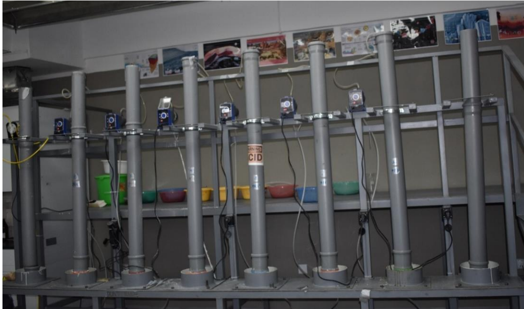
Figure 15: PVC leaching columns
