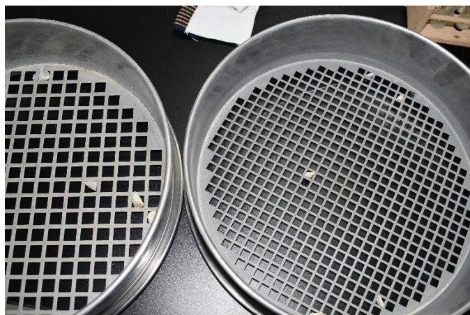
Figure 14: 19&12.5mm size sieves
