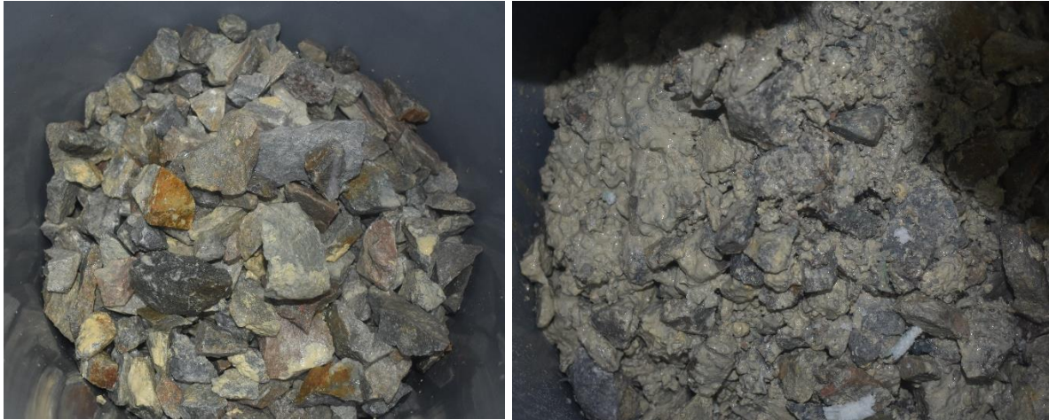
Figure 21: Mixed and >19mm size fraction leaching residues after leaching
