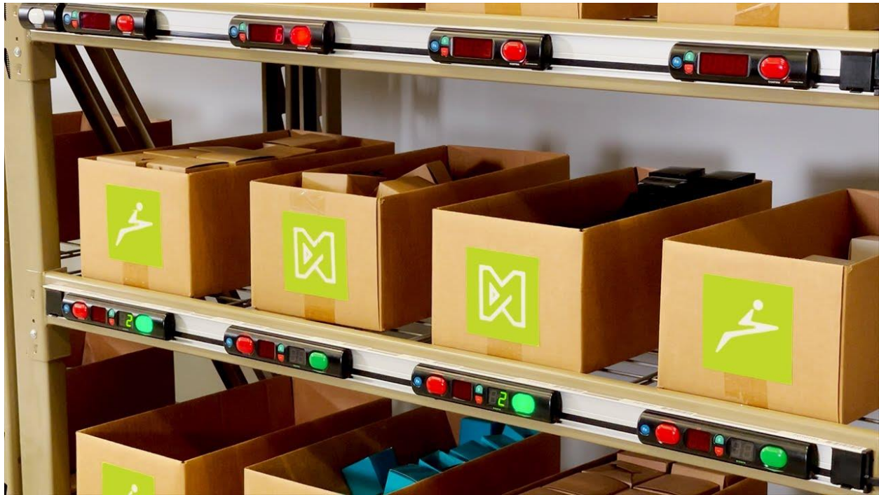
Figure 2.7: Pick-to-Light system, LED display in use.
