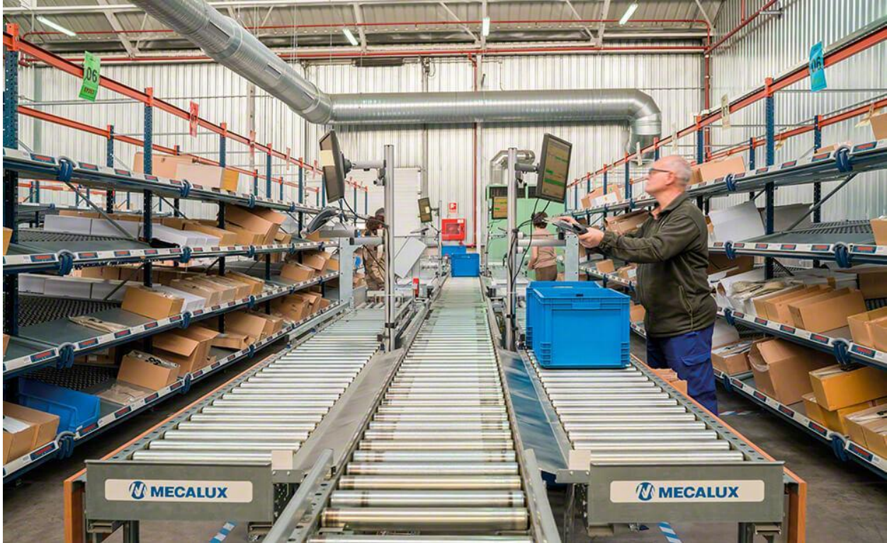
Figure 2.8: Pick-to-Light system and conveyor in use.
