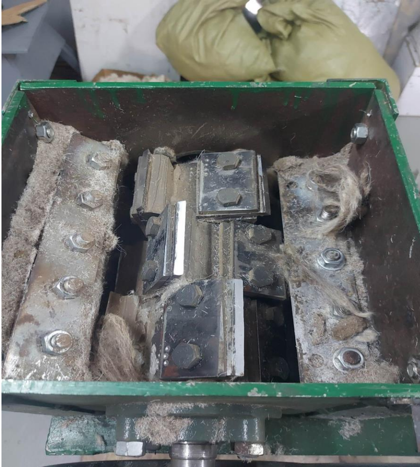
Figure 29. Blades in shredding chamber
