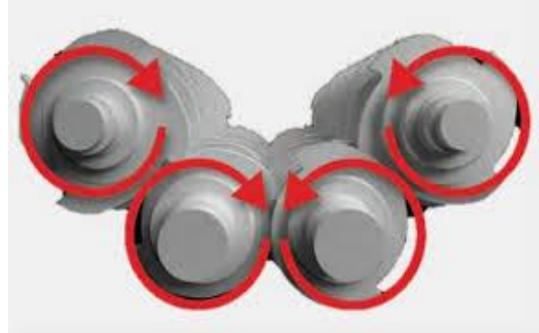
Figure 13. Four shaft shredder
