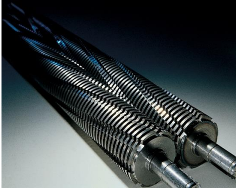
Figure14. Cross-cut blades of shredder
