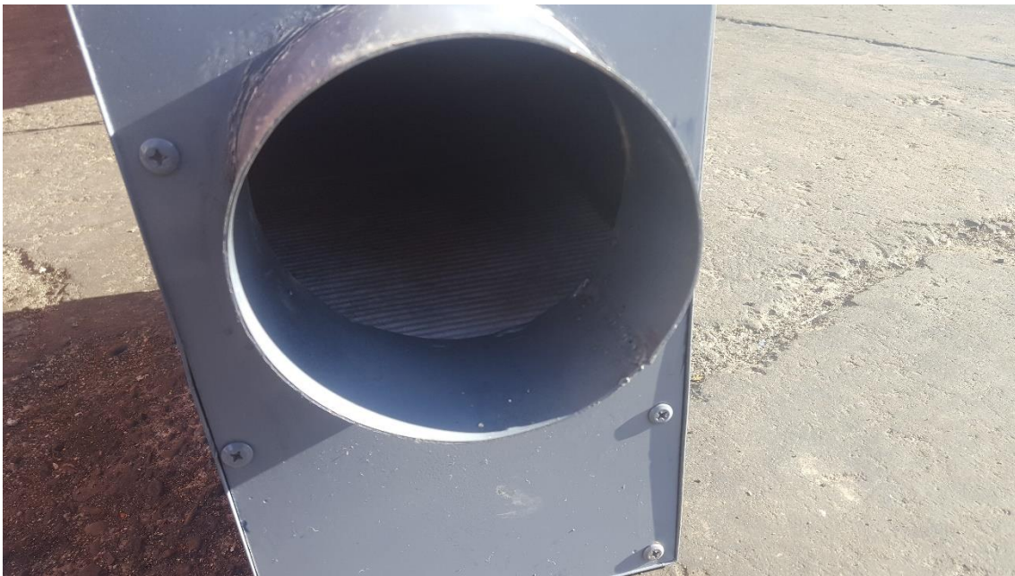
Case inlet of the air with the activated carbon air filter
