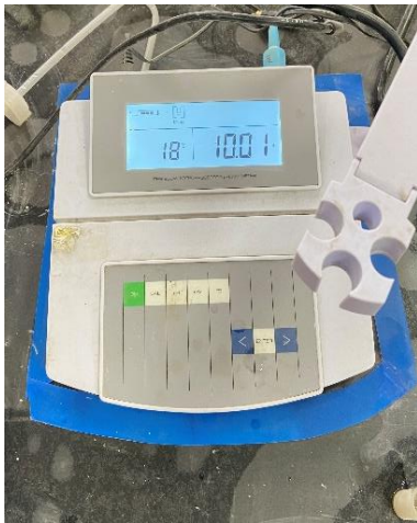
Figure 27: Measurement of pH by using the PHS-25CW microprocessor pH/mV
