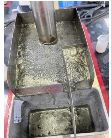
Figure 29: Froth scalping during the rougher flotation
