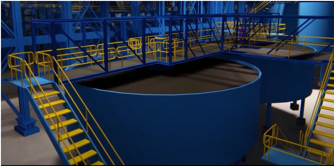
Figure 7: Concentrate dewatering at Oyu Tolgoi concentrator [4]
