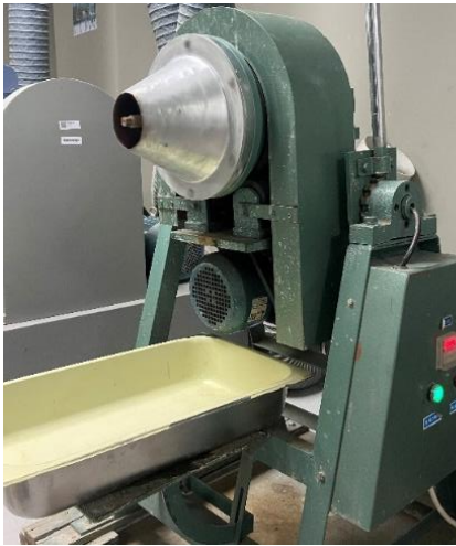
Figure 19: Laboratory rod mill
