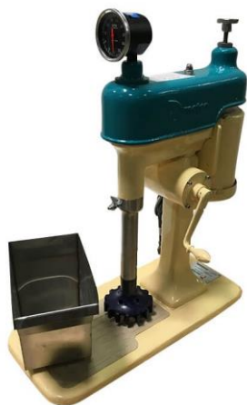
Figure 33: Metso D12 Laboratory Flotation Machine [7]
