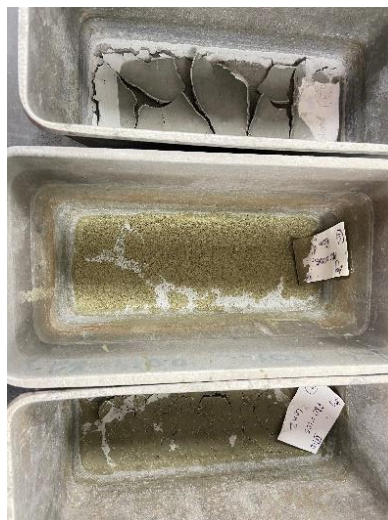
Figure 31: Concentrate of 1,2 & 3 after drying oven
