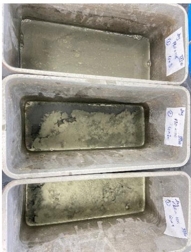
Figure 30: Concentrate 1,2 & 3 after rougher flotation
