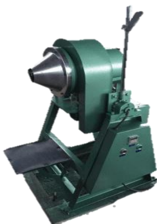
Figure 34: XMB laboratory rod mill [8]
