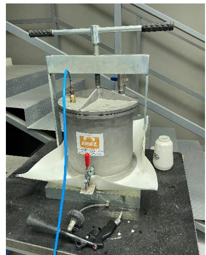
Figure 32: Dewatering slurries by using the MACSALAB Filter Presses
