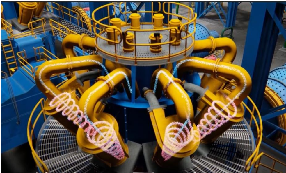
Figure 5: Hydro cyclone of Oyu Tolgoi concentrator [4]
