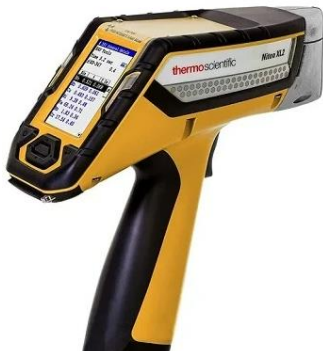
Figure 37: The Thermo Scientific Niton XL2 XRF Analyzer [13]
