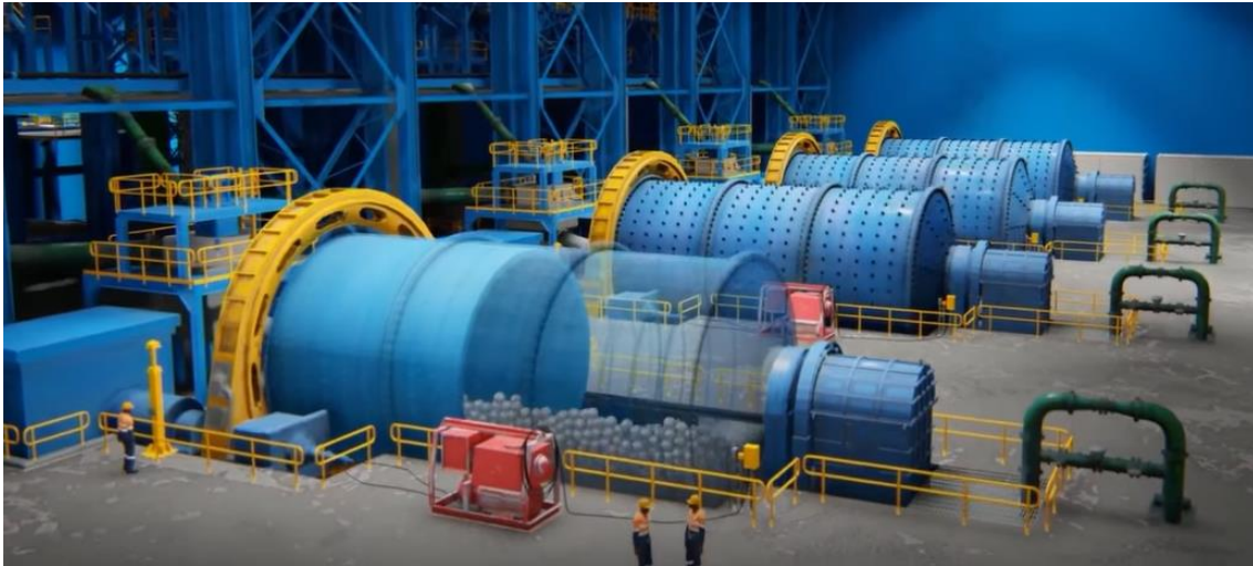
Figure 4: The ball mill of Oyu Tolgoi concentrator [4]
