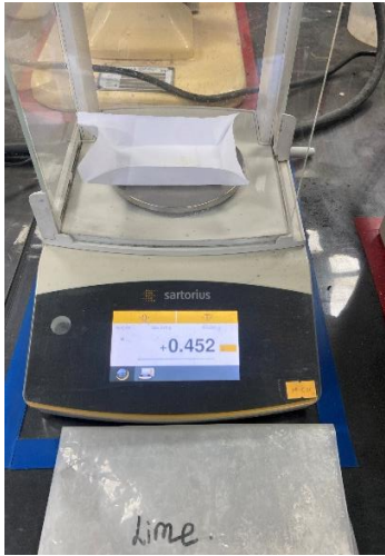
Figure 24: Weighing the lime as a conditioner on the laboratory balance
