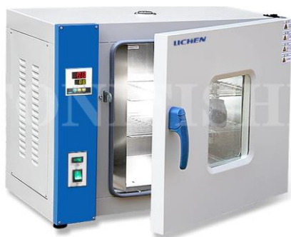
Figure 40: Lichen technology electric blast drying oven [15]
