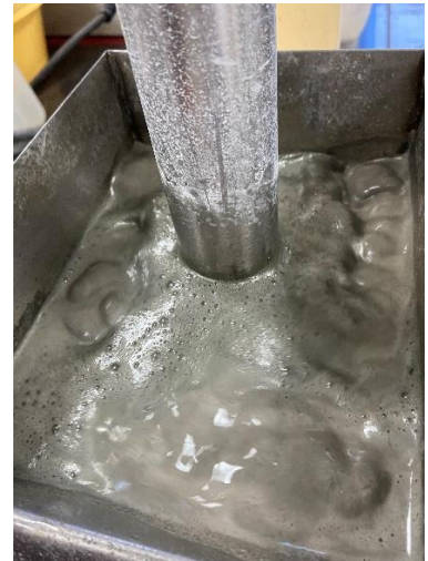
Figure 26: Rougher flotation conditioning
