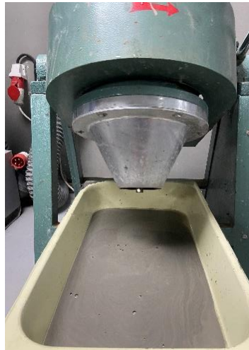
Figure 20: Slurry as a output of the rod mill
