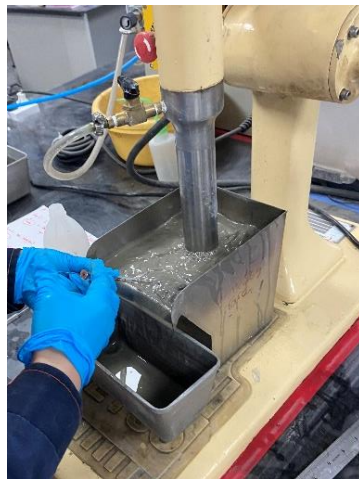
Figure 28: Addition of collector & frother prior to the rougher flotation
