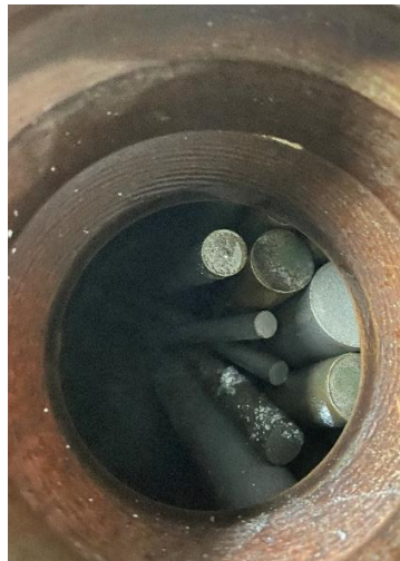
Figure 25: Rod mill inside before experiment
