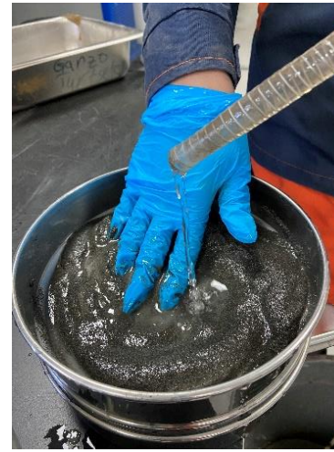
Figure 21: Particle size analysis with wet method
