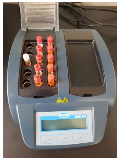
Figure 12 Digital Reactor Block DRB 200 (Author)
