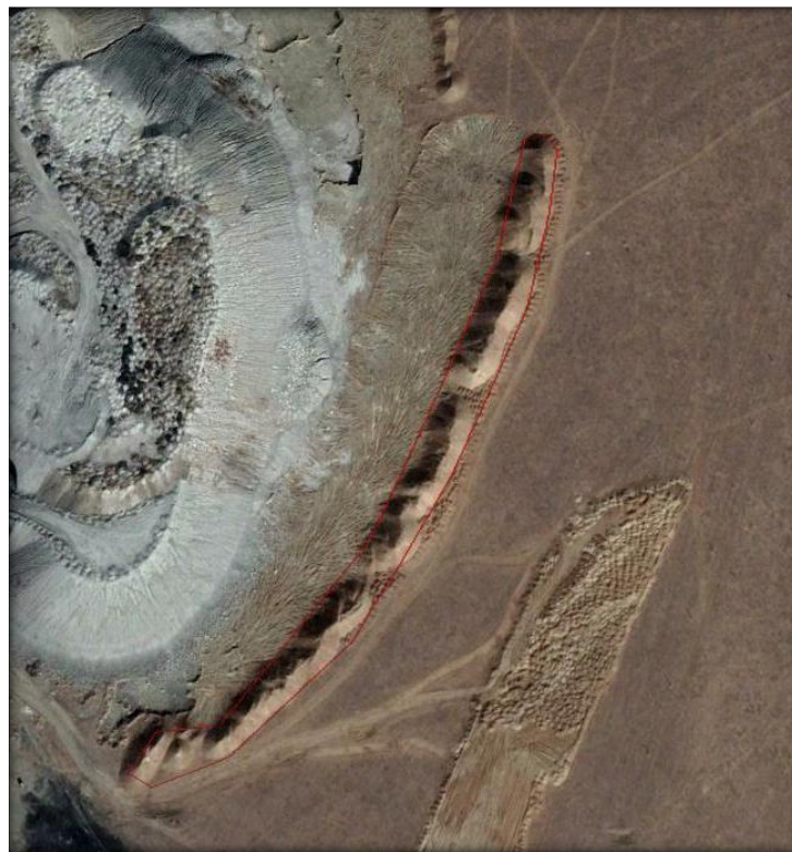
Figure 10. Dirt piles used to prevent sediment washing from the Baganuur mines waste tips.
