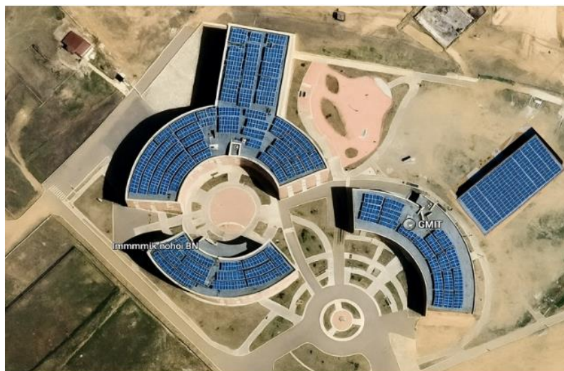
Figure 12 Solar Collector Placement
