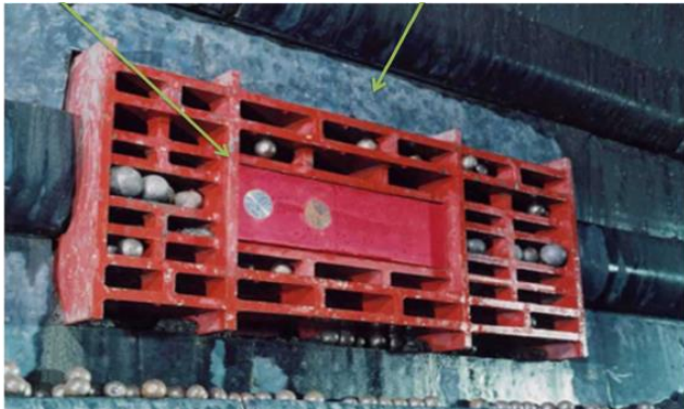
Figure 2. 17 – Example of Polyurethane Sensor Beams inside of mill shell
