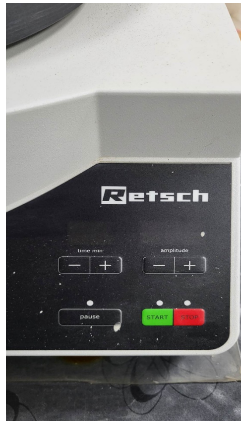
Figure 15 / Controller of automatic sieve apparatus/
