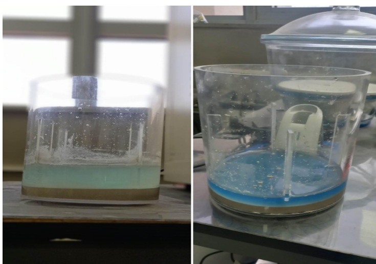
Figure 20 /Color comparison of 0.1M sulfuric acid leaching solution and 0.1M glycine leaching solution/
