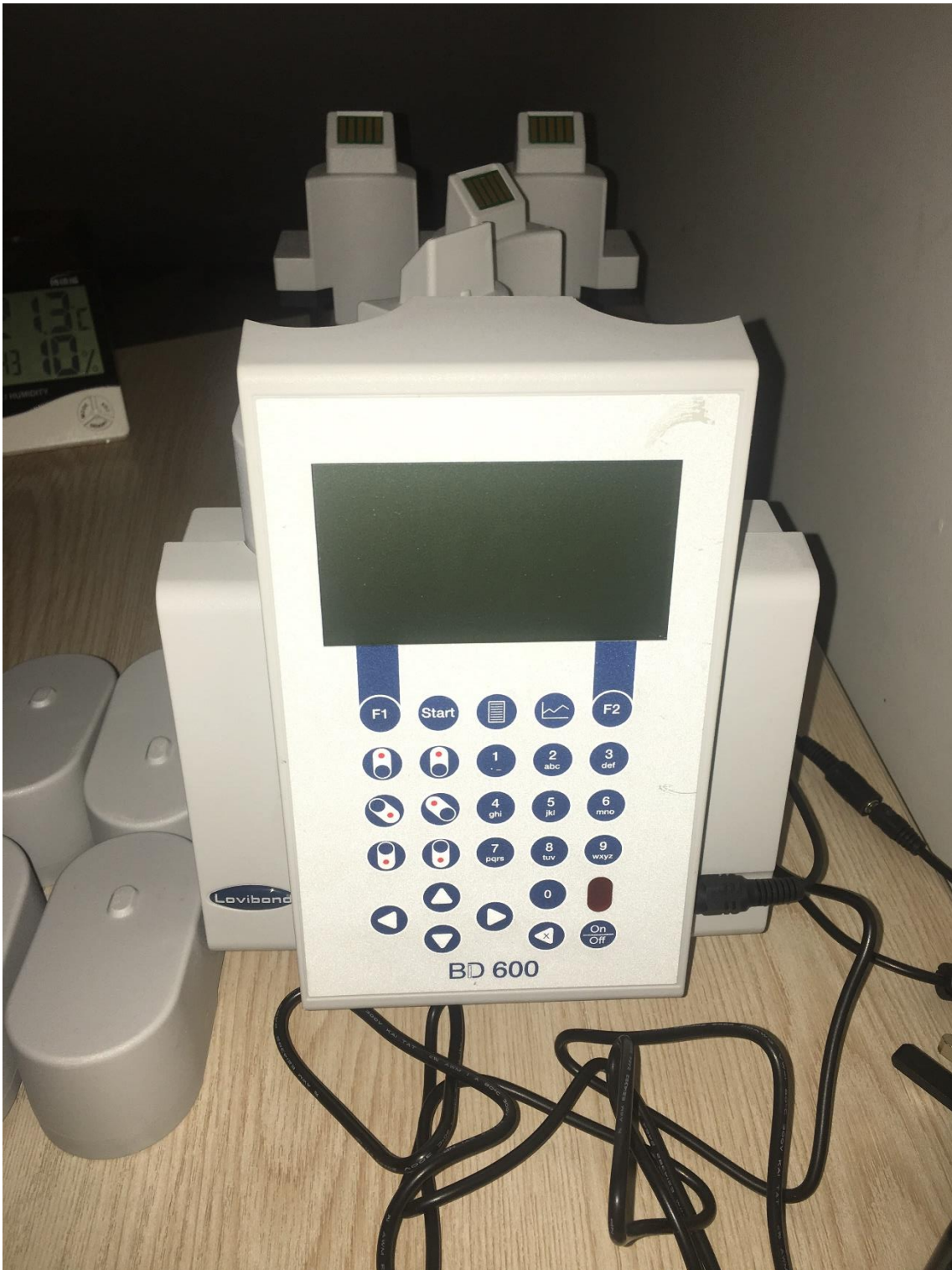
Figure 5: The Lovibond BOD-System BD 600 used for BOD Measurement
