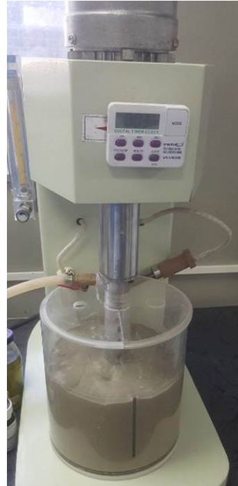
Fig. 4.6: Vat leaching tank and mixer
