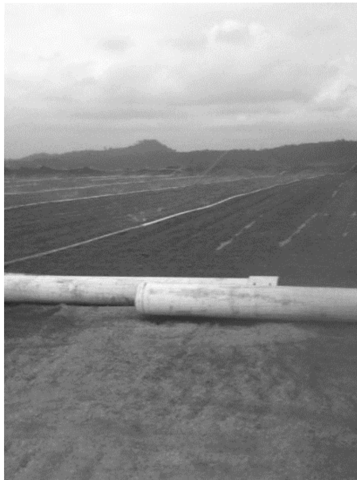
Fig. 2.6: Examples of heap leaching operations[6].
