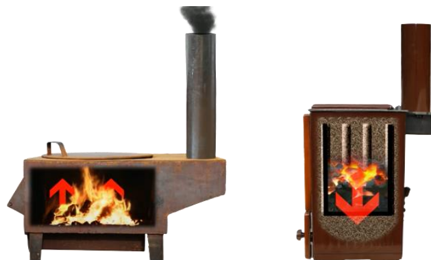
Figure 3: Differences in Combustion between Traditional Stove and Millennium Challenge Account Stove
