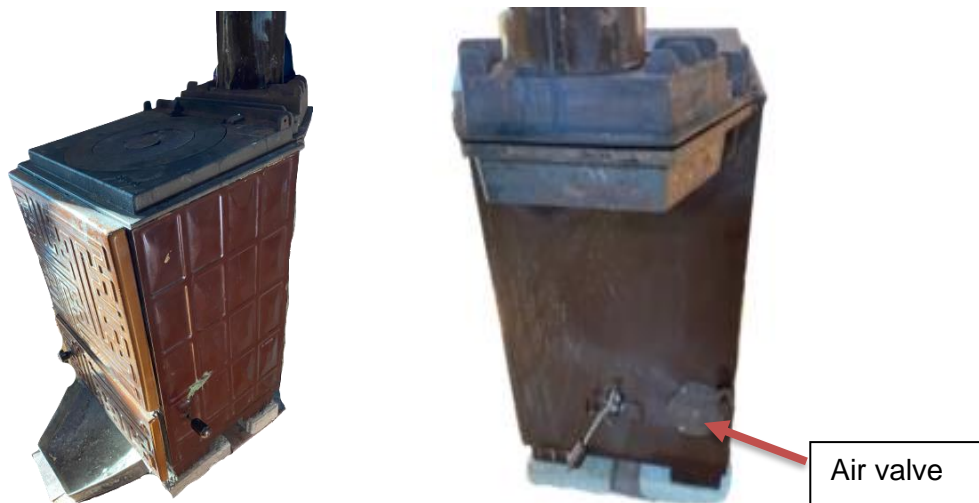
Figure 4: a) Isometric view of the Ulzii stove b) The back view of the Ulzii stove.
