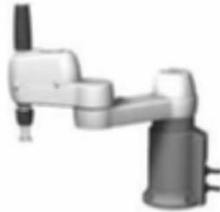
Fig. 2.6 A SCARA Robot designed for assembly.
