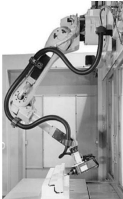
Fig. 2.7 Articulated robots used in machining, spray painting, welding etc.
