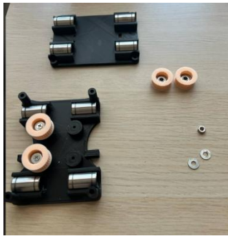
Figure 31: Fixed bearings and pulleys
