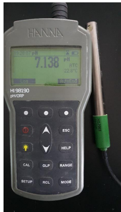
Figure 10. Hanna pH/ORP waterproof portable meter
