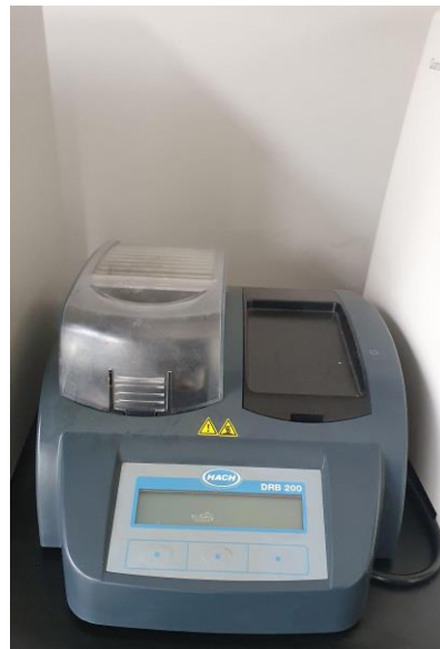
Figure 8. Digital Reactor Block DRB 200
