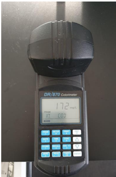
Figure 7. Hach DR/870 Colorimeter
